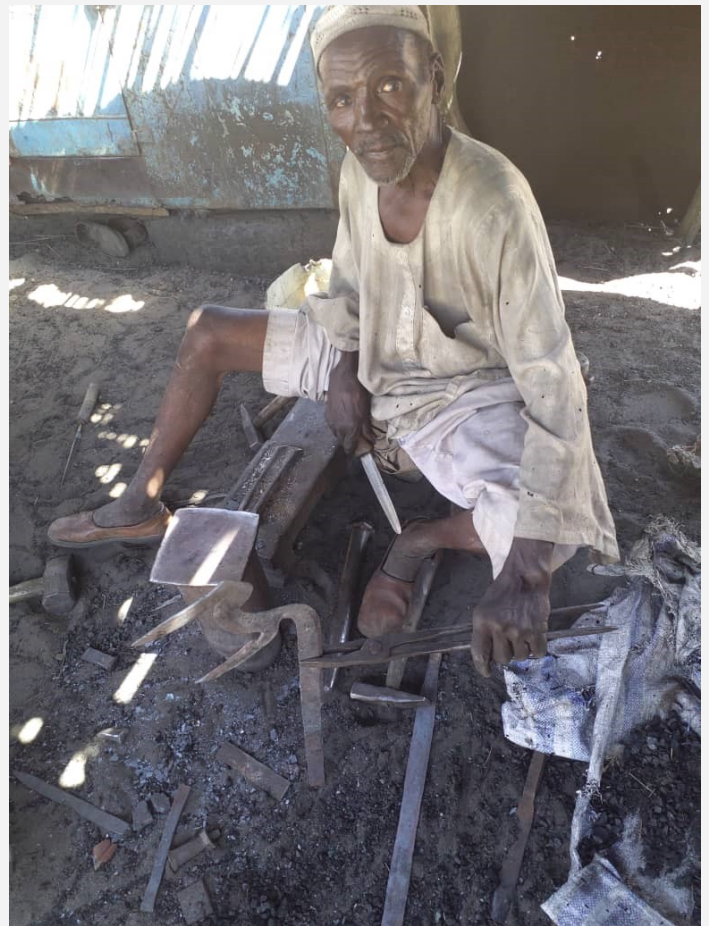
Figure 1: Forging Farming Tools—Two pronged hoe called Najjama
